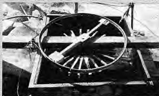
Turbine with bike dynamo at left.
