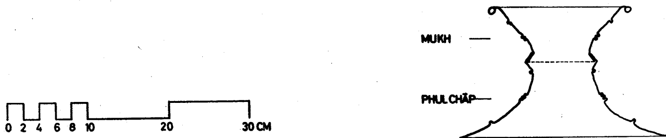
Fig. 8: The gāgri. Joining mukh and phul chāp.
