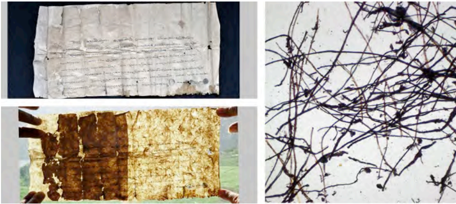
Figs. 32 a, b, c. Document LT/23 from Lower Tshognam written on paper made of Daphne/Edgeworthia sp. fibres. a. Recto side of the document; b. Paper transparency observed against light; c. Fibres observed in 50× magnification.
