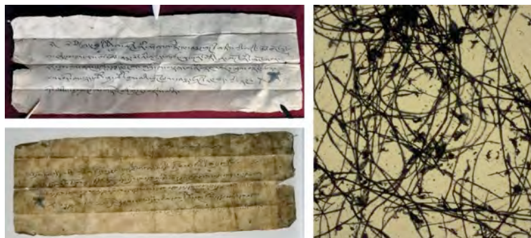
Figs. 22 a, b, c. Document UT/06 from Upper Tshognam written on paper made of pure Daphne/Edgeworthia sp. fibres. a. Recto side of the document; b. Paper transparency observed against light; c. Fibres of Daphne/Edgeworthia sp. observed in 50× magnification.
