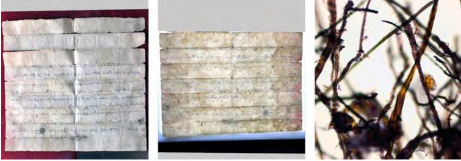
Figs. 35 a, b, c. Document UT/05 from Upper Tshognam written on paper made of mixed fibres of Daphne/Edgeworthia sp., Stellera sp. and other recycled fibres. a. Recto side of the document; b. Paper transparency observed against light; c. Fibres observed in 200× magnification.
