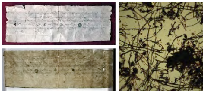
Figs. 15 a, b, c. Document UT/02 from Upper Tshognam written on paper made of Daphne/Edgeworthia sp. fibres with small addition of Stellera sp. fibres. a. Recto side of the document; b. Paper transparency observed against light; c. Fibres observed in 50× magnification.
