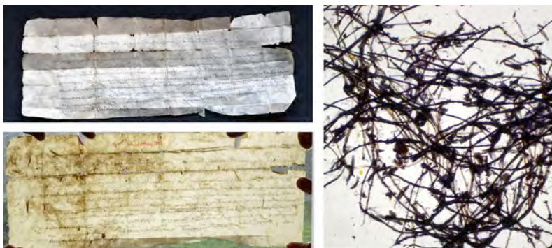
Figs. 30 a, b, c. Document LT/11 from Lower Tshognam written on paper made of mixed fibres of Daphne/Edgeworthia sp., Stellera sp. and individual synthetic fibres. a. Recto side of the document; b. Paper transparency observed against light; c. Fibres observed in 50× magnification.
