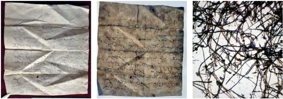
Figs. 44 a, b, c. Document UT/39 from Upper Tshognam written on paper made of Daphne/Edgeworthia sp. fibres. a. Recto side of the document; b. Paper transparency observed against light; c. Fibres observed in 50× magnification.
