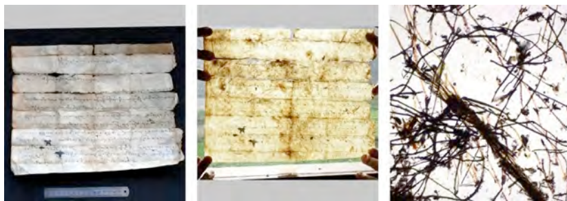
Figs. 33 a, b, c. Document LT/04 from Lower Tshognam written on paper made of Daphne/Edgeworthia sp. fibres. a. Recto side of the document; b. Paper transparency observed against light; c. Fibres observed in 50× magnification.
