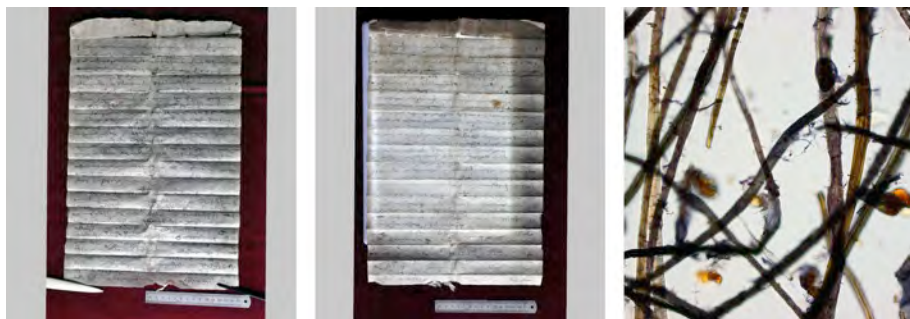
Figs. 38 a, b, c. Document UT/33 from Upper Tshognam written on paper made of mixed fibres of Daphne/Edgeworthia sp., Stellera sp. and other recycled fibres. a. Recto side of the document; b. Paper transparency observed against light; c. Fibres observed in 200× magnification.
