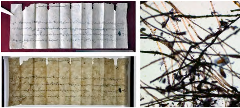
Figs. 28 a, b, c. Document UT/34 from Upper Tshognam written on paper made of mixed fibres of Daphne/Edgeworthia sp., Stellera sp. and other recycled fibres. a. Recto side of the document; b. Paper transparency observed against light; c. Fibres observed in 100× magnification.
