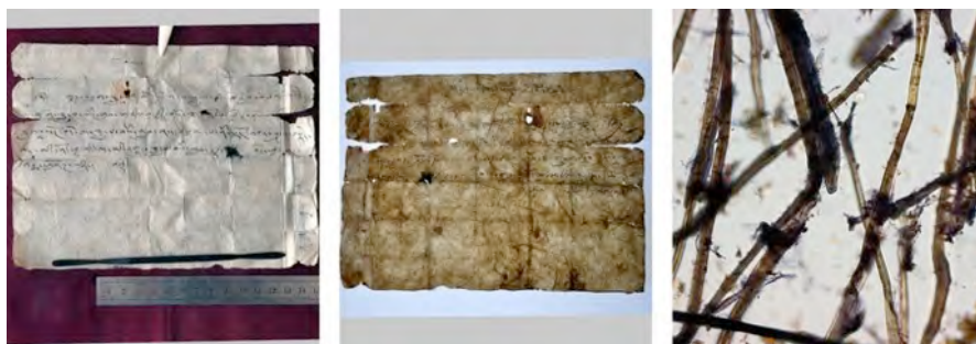
Figs. 24 a, b, c. Document UT/09 from Upper Tshognam written on paper made of Stellera sp. fibres with small addition of Daphne / Edgeworthia sp. fibres. a. Recto side of the document; b. Paper transparency observed against light; c. Fibres observed in 200× magnification.
