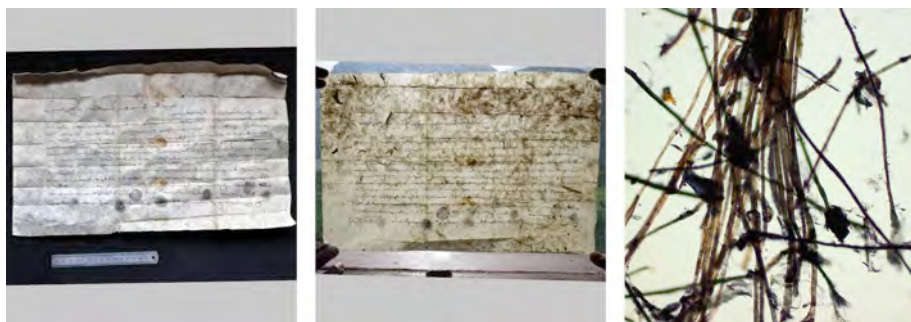
Figs. 11 a, b, c. Document LT/17 from Lower Tshognam written on paper made of pure Daphne/Edgeworthia sp. fibres. a. Recto side of the document; b. Paper transparency observed against light; c. Fibres of Daphne/Edgeworthia sp. observed in 100× magnification.
