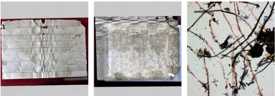
Figs. 19 a, b, c. Document UT/24 from Upper Tshognam written on paper made of pure Daphne / Edgeworthia sp. fibres. a. Recto side of the document; b. Paper transparency observed against light; c. Fibres of Daphne / Edgeworthia sp. observed in 100× magnification.
