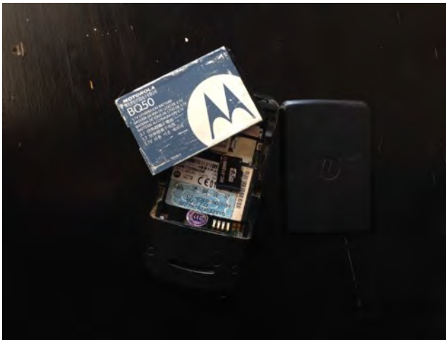
Fig. 5 - Example of a 512 MB Micro SD that could be inserted into flip phones as external storage. Photo by Kati Fitzgerald December 3, 2016.
