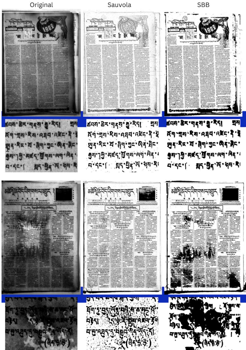
Figure 4 A visual comparison of baseline (lightly treated) images, their counterparts treated with Sauvola and SBB binarisation 7
