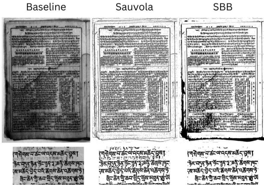
Figure 13 Sauvola binarisation used hyperparameters ( k -value and window size) optimised for all three test subsets (fair-quality, poor-quality, red text) - the trade-off resulted in poorly binarised bleed-through relative to SBB binarisation (Qinghai Tibetan News, Jul. 12 1952 p2).
